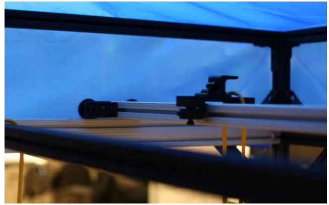
Figure 4: Horizontal sliders move in the XY plane as the user moves their arms to mimic a swimming gesture. The sliders are attached to resistance bands (in yellow), which are attached to user's arms and legs.
